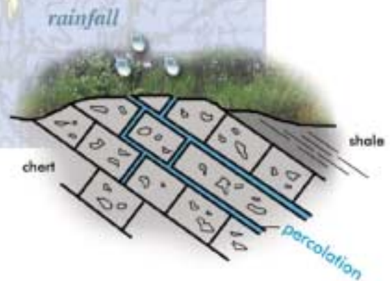
Fig. 4. Where the fractured Fort Payne Chert is exposed, water entering cracks and moving along fractures recharges the aquifer. When this water becomes contaminated, the aquifer and its water resources are at risk.
